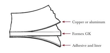
Note: Formex GK, Formex GL, Formex N3 and Formex GS materials have been specifically produced to accept adhesives. Adhesive performance will be improved by maintaining surface cleanliness. Pure isopropyl alcohol may be used for this purpose if required.
