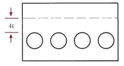
A series of holes must be kept at a minimum distance from a score line to prevent the part from folding through the holes. Four material thicknesses is the recommended minimum.
