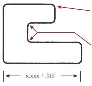
Rounded external corners increase die strength and service life. Additional benefits include faster production, prevention of cracks, corner splits and burrs.
