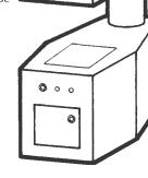
AUTOMATIC PRESS Operator not always required; feeds and cycles automatically. Cuts steel to steel for good depth accuracy. Primarily uses roll stock, good for high volume runs, can count and prepackage parts.
