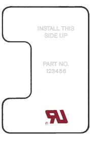
Note: Formex GK materials have been specifically produced to accept printing inks. If product has become dirty during fabrication, printing quality can be maintained by cleaning the part with pure isopropyl alcohol prior to printing.
